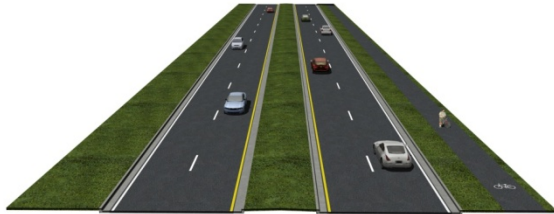
Figure 9. Four-Lane Median-Divided Alternative Typical Cross-Section
